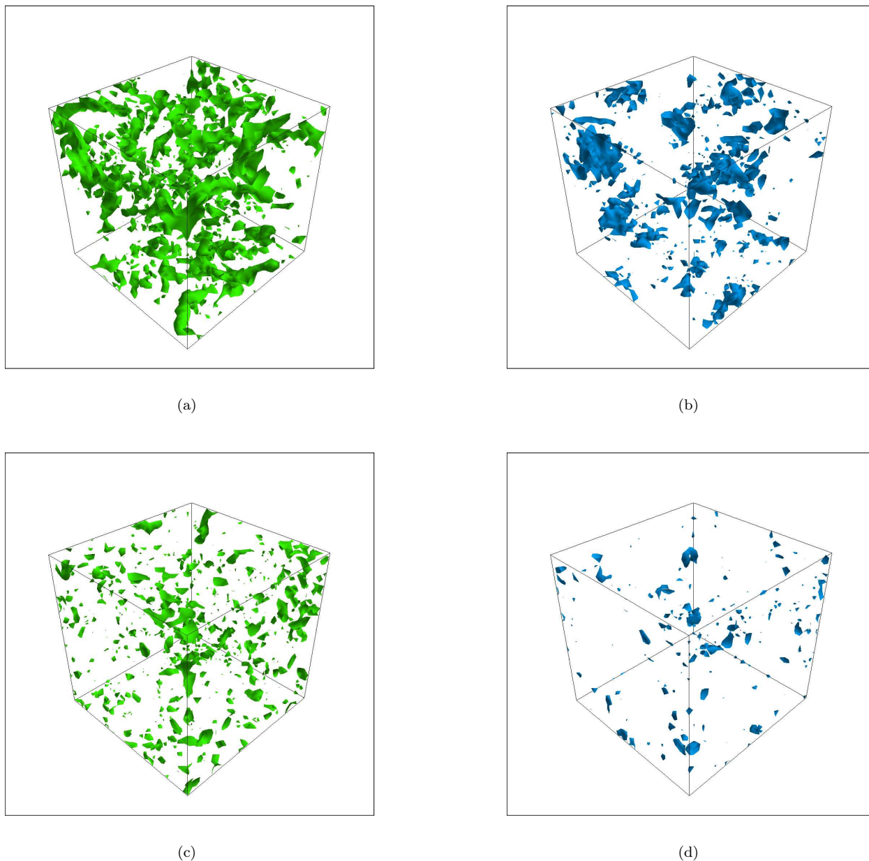
Figure 13. Decay of isotropic turbulence: the LS (a, c) and the resolved SS (b, d) vorticity magnitude isosurfaces at the same intensity level for two instants of time T = 0.75 and 3.
