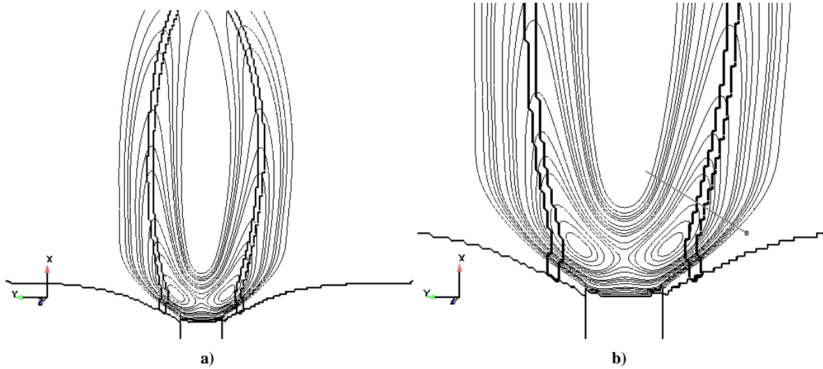
Figure 10 (a) The structure of APd-binder flame. The double line is stoichiometric mixture and the contours are reaction rates for APd/binder reaction rates; (b) Detail: The line is the limit between diffusive and premixed flames.
