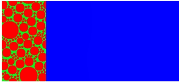
Figure 13 Computational domain for random packing (the circles are AP particles with binder in between, the dark color is the gas phase). The package consists of AP particles of 10, 30, 40 and 80 \mu\text{m} embedded inside a binder.
